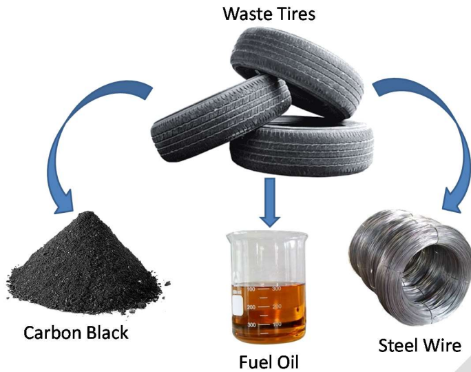
Figure 7. Products from the pyrolysis of waste tires.
