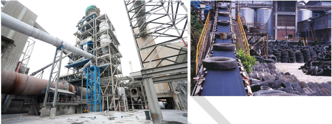
Figure 5. Tires sent for co-processing at the Golden Bay Cement Works where both fuel value and materials are recovered.
