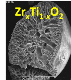
Ceramic with hierarchical porosity
